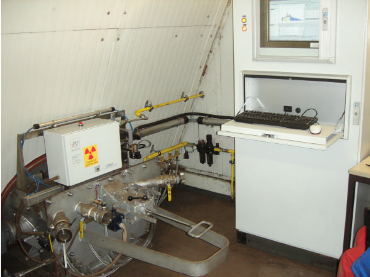
Fig 8: Online Zinc measurement of converter dust
