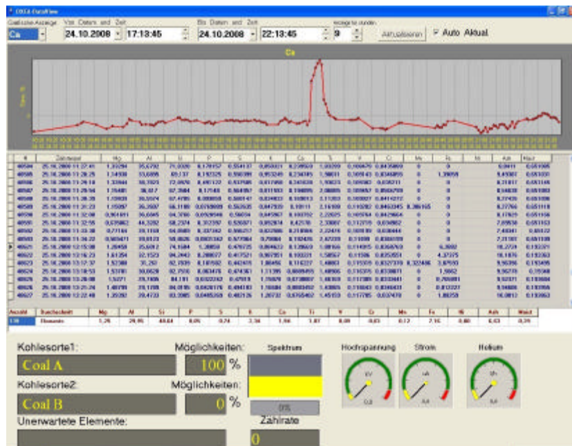
Fig. 15: Type recognition screen in the control room
