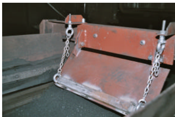
Fig. 5: Hinged plate to smooth the surface of the coal.
