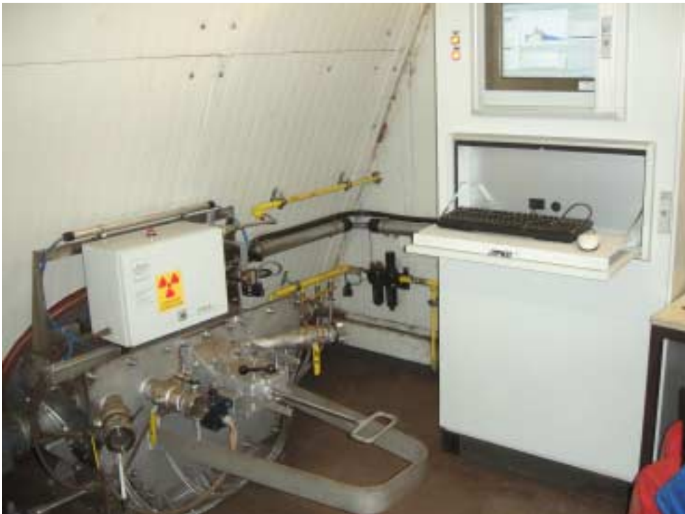
Fig. 9: Online Zinc measurement of converter dust
