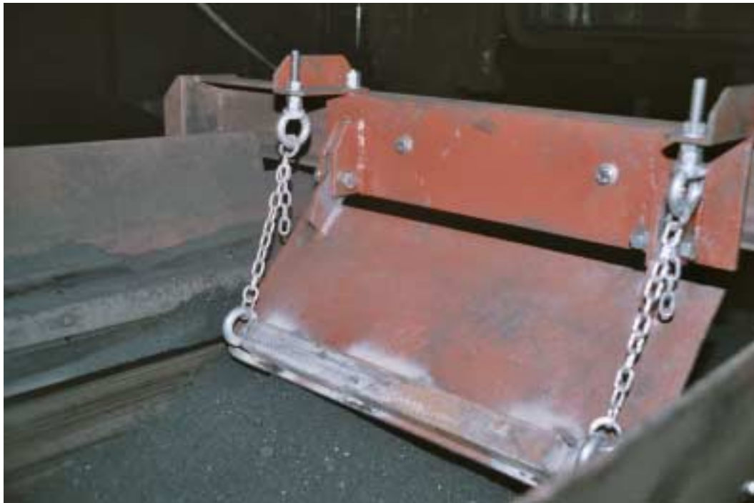
Fig. 4: Hinged plate to smooth the surface
